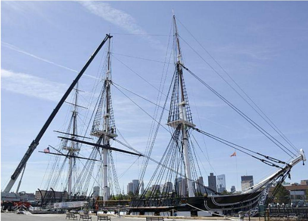
180531-N-SM577-0136 BOSTON (May 31, 2018) Ship's riggers assigned to Naval History and Heritage Command, Detachment Boston, raise USS Constitution's main mainmast yard back into place. The square-rigged frigate is America's Ship of State and the oldest commissioned warship afloat in the world. (U.S. Navy photo by Mass Communication Specialist 3rd Class Casey Scoular/Released)
