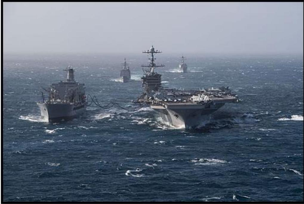
180510-N-UD522-0269 PACIFIC OCEAN (May 10, 2018) The aircraft carrier USS John C. Stennis (CVN 74), right, conducts a replenishment-at-sea with the fleet replenishment oiler USNS Henry J. Kaiser (T-AO 187). John C. Stennis is underway with the ships and squadrons of Carrier Strike Group (CSG) 3 conducting a group sail training in preparation for its next scheduled deployment. (U.S. Navy photo by Mass Communication Specialist 2nd Class David A. Brandenburg/Released)
